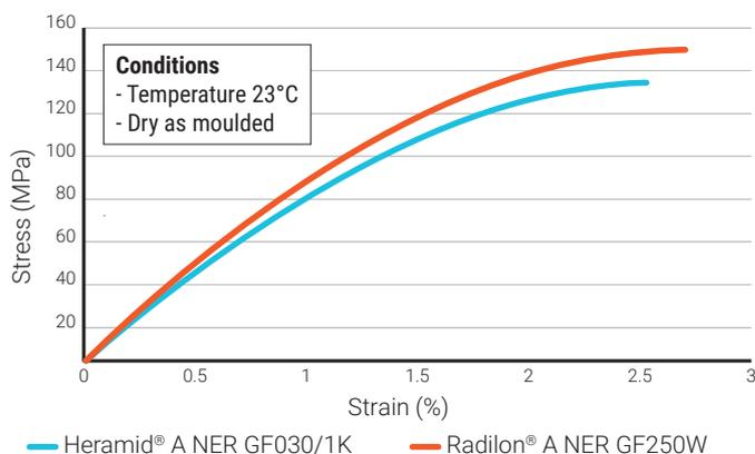
Figure 8: Stress-strain curve
