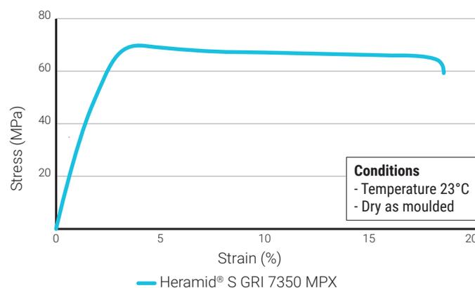
Figure 17: Stress-strain curve
